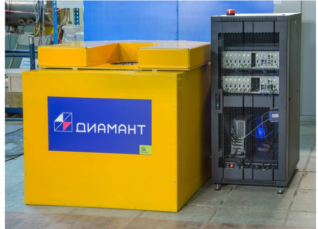
Figure 2. General view of the neutron module and the electronics cabinet of the AGP-F analyser.
