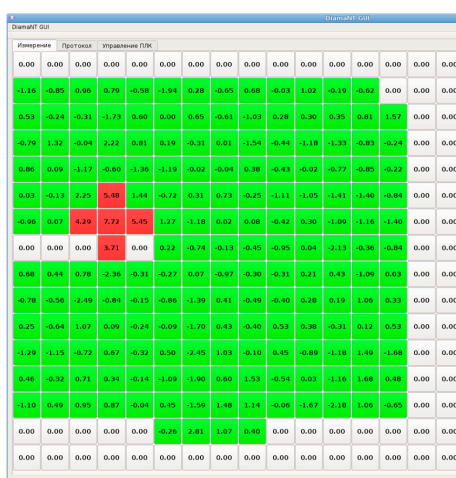
Figure 9. The operator interface for irradiation of 20 mm imitator inserted inside the -90 mm kimberlite stone. In grey colored cells there is no enough statistics to calculate the carbon concentration, the green colored cells depict carbon excess less than 3\sigma , the red ones show carbon excess larger than 3\sigma .
